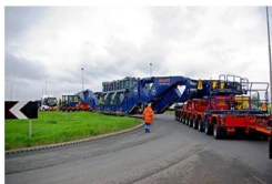
Image of a transformer being delivered to site on the abnormal indivisible load (AIL) vehicle. nationalgrid.com/news/electricity/transformer-repairs/athens-substation
